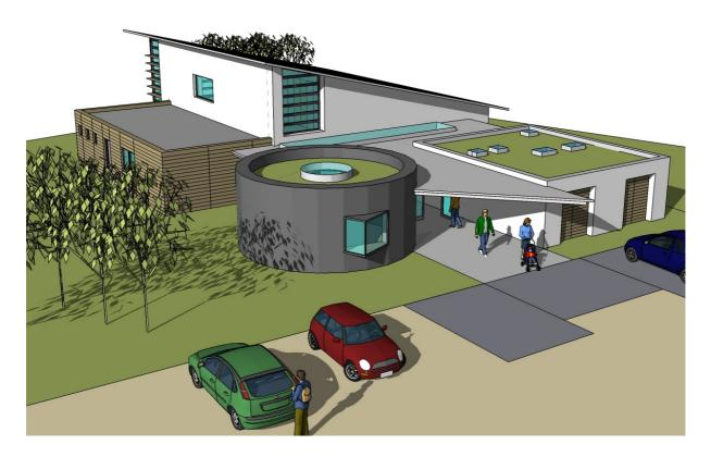
The main hall and meeting room will be built using timber frame and straw bales, suitably rendered and clad to make them weather-proof. The flat roofs will be 'living roofs' planted with Sedum or other appropriate plant life. Other eco design features are still under evaluation.
